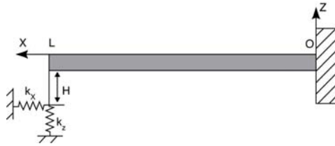
FIGURE 3 AFM cantilever scheme. The lever is embedded at x=0 and the length is L . The tip is positioned at x=L-\delta x . The contact stiffness is represented by two springs, one for the vertical displacement and the other for the lateral.
