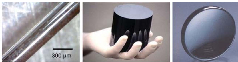
FIGURE 6 Examples of optical elements made of chalcogenide glass. The outstanding rheological properties permit to produce large optics or to shape the glass into fiber and molded lenses.
